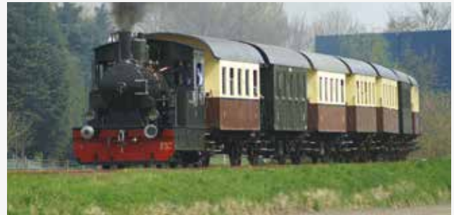
Coaches 51-61 & 86 have been built by railway companies in the early fifties on underframes dating back to the early 1900s; they were acquired by the SHM and have seen almost daily use since 1975. Their design closely resembles the four-wheeled coaches which were in use throughout the Netherlands on rural branch lines, including the one to Medemblik. The redbrown coach nr. 86 was built for the transportation of Dutch coalmine workers in 1917.
